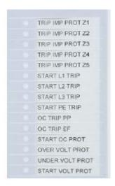
Fig. 6 Trip indication LEDs
